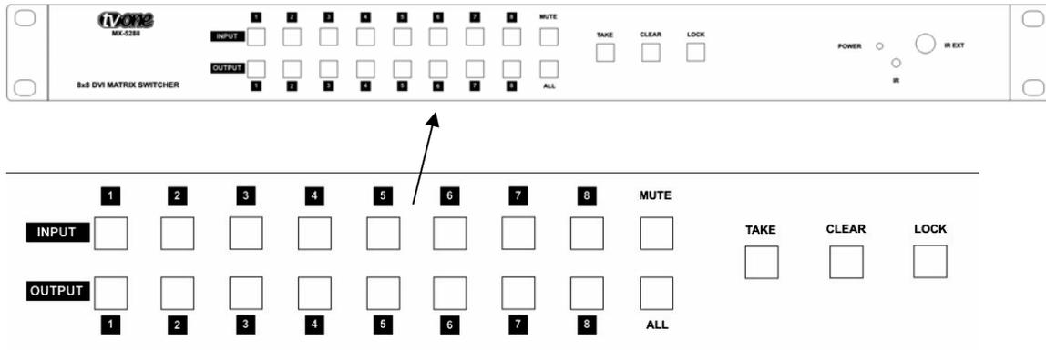
There are eight input and eight output selectors, a “Mute” button, a “Take” button, A “Clear” button, a “Lock” button and a button labeled “All”.
