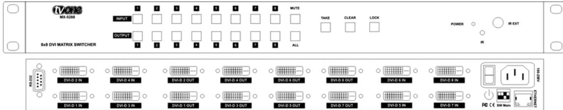
The MX-5288 is an 8x8 DVI-D Matrix Switcher capable of switching non-HDCP encrypted DVI digital video.
