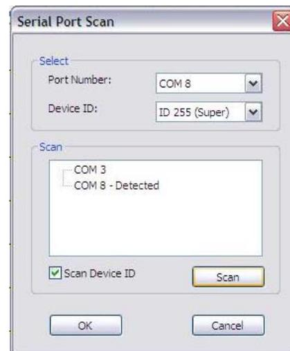
*Note: Selecting Device ID 255(Super) will cause the software to send commands that will affect units with any Device ID on the selected COM port.*
