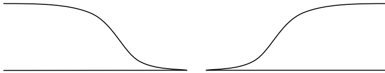
S-curves for left and right projectors, with edges blended.
