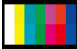
Color Space Comparison (Simulation): The top part shows the color space when set to the ITU-709 mode. The bottom part shows the color space in the WIDE3 (D-Cinema) mode. This screen image is simulated to show the differences in colors
