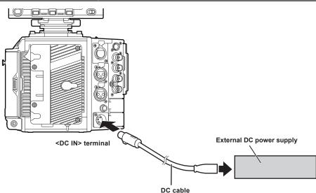
**1** Connect the external DC power supply to the <DC IN> terminal of the camera.
