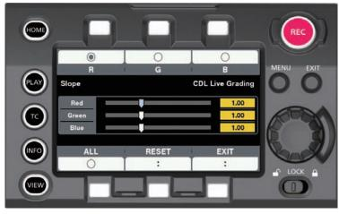
Various parameters can be adjusted from this screen when [Grading SEL] is set to [Internal]. This can be adjusted in 0.01 steps with the control panel operation button. It is reflected to video in real time.
