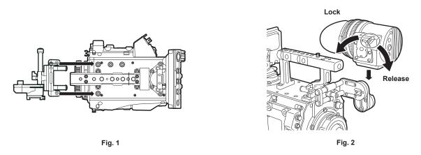
1 Attach the slider unit to the viewfinder mounting holes on top of the camera using the two supplied screws. (Fig. 1)
