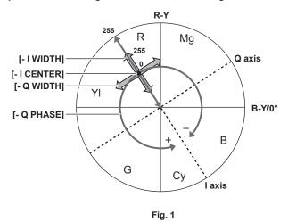
The color composition of video signal (R/G/B) can be converted to color difference signal (R-Y/B-Y) as in (Fig. 1).
