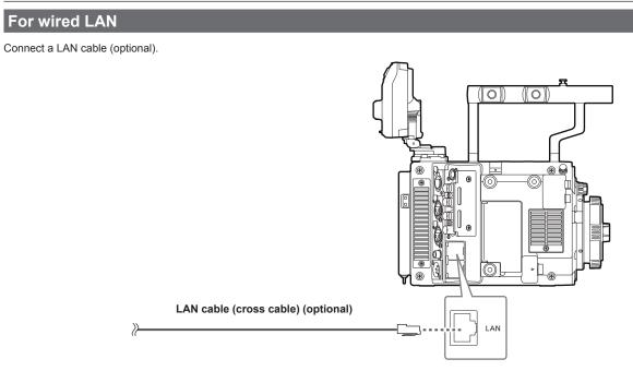
1 Connect the LAN cable to the <LAN> terminal on the right side.
