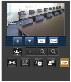
When this button is pressed, the buttons for performing the camera menu operations are displayed on the screen. At the same time, the camera menus are also displayed on the monitor images of the unit.
