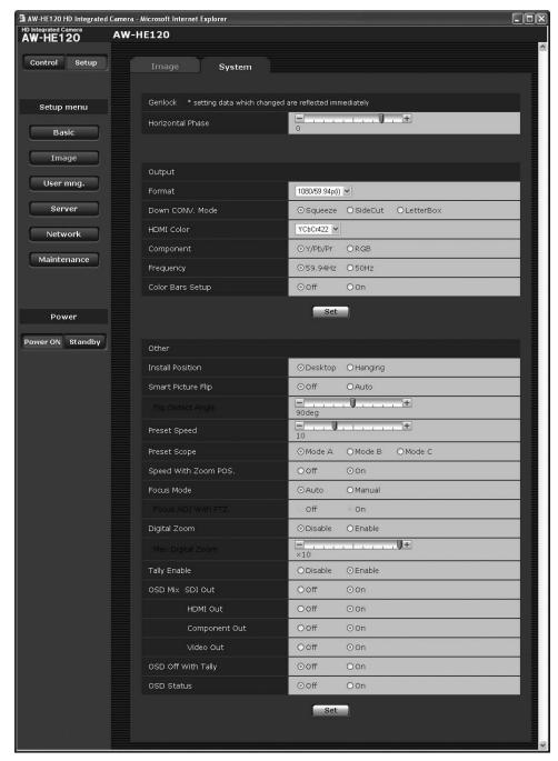
(The screen displays when the unit's frequency has been set to 59.94 Hz.)
