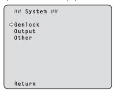
4 Press the [▲] or [▼] button to bring the cursor to "Genlock", and press the [○] button.
