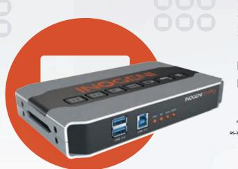
The unit features a HDMI and a DVI-I input, stereo audio input, stereo audio output, internal USB 3.0 hub with 2x USB ports for expansion purposes and a USB host connector. It supports SD/HDTV video formats up to 1080p60 and most computer graphic formats. SHARE2 comes with a USB 3.0 cable, DVI to VGA and DVI to HDMI adapters.
