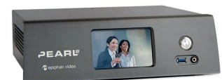
Epiphan Pearl 2 is a 6-input recorder and streamer with a touchscreen interface
