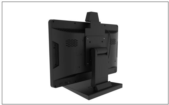
Aline the 4 screws holes at the back of TAURI to FIX-028 Table Stand screw positions, and place screws to fixate it.
