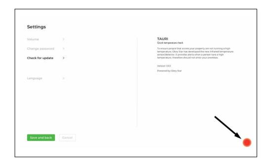
2.4 To get connected to **WIFI**, press the bottom right corner 4 times and enter" 0000" to exit TAURI.
