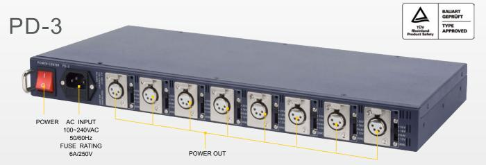
The Datavideo PD-3 is a 19" rack mountable universal AC to DC power distribution center, designed to supplies a steady user chosen voltage for production kit whilst on location or in your studio.
