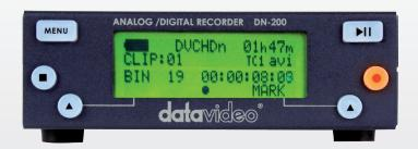
The Datavideo DN-200 is a small portable hard drive based video recorder, capable of analogue, DV & HDV recording.
