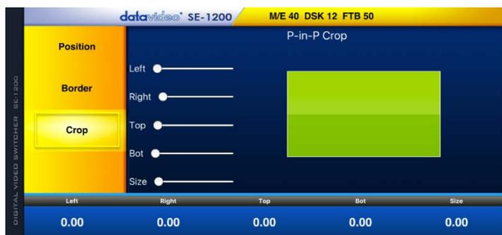
The **Left**, **Right**, **Top** and **Bottom** edge values of the crop can be adjusted individually or together using the **Size value**. Click on a single value to adjust just that edge of the PIP.
