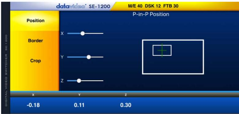
**Step 6:** PiP options displayed in the yellow menu area: **Position**, **Border** and **Crop**. The sections below will describe how Position, Border and Crop can be adjusted.
