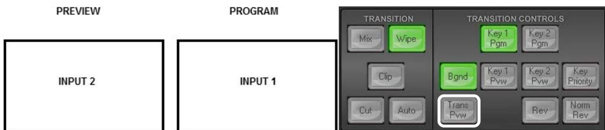
Using the **TRANSITION CONTROLS** panel click to select the **Trans Pvw** button (back lit green is ON). Next select and apply the transition or wipe that you would like to test on the Preview monitor.
