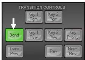
In order to enable clip transition between two video sources first ensure the Background Transition or **Bgnd** button is ON / backlit green in the **transition controls** area of the user interface.
