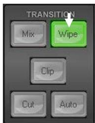
Clicking **Wipe** will select the current wipe transition in use when moving from the current video source on the Program row to the selected next source on the Preset row.
