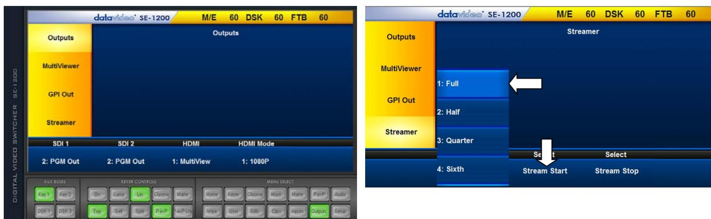
By choosing HALF instead of FULL you are using less bandwidth to support the multi view stream being sent across the IP network.
