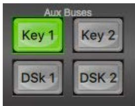
The SE-1200 MU has four dedicated keyers, **Key1, Key2, DSK1** and **DSK2**. All four keyers can be active simultaneously. **Key 1** and **Key2** can be set as Upstream or Downstream keyers.
