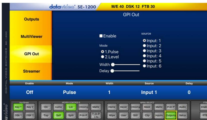
This feature could be used to trigger playback from units such as the DataVideo **NVP-20** or **HRS-30** or **HDR-60/70**.
