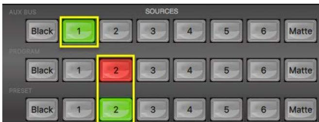
**Step 3:** Select the **foreground video** source with the subject or talent to be keyed. In our example, we want to use a green screen source connected to **Input 1** on the **Aux Bus Row**.
