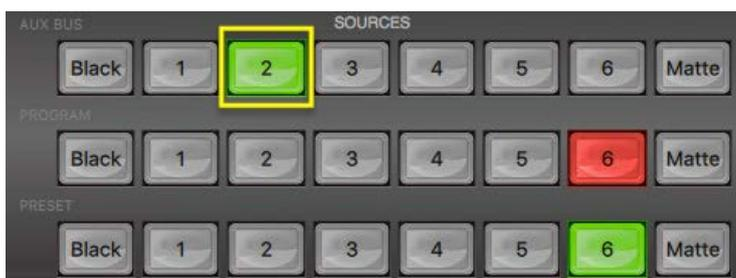
**Step 4:** Select the PiP image source on the **AUX BUS** row of the **SOURCES** panel. This will be shown over the chosen Preview image before being taken to Program/air with the next mix or wipe transition.
