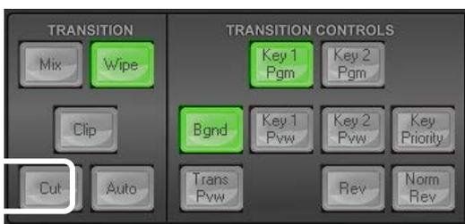
When the **Nrm / Rv** button is **ON**, the selected WIPE transition will automatically switch directions as each transition is completed. The **Rev** button will switch on and off automatically to indicate the direction of the next transition.
