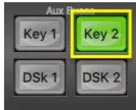
**Step 1:** Choose the desired Keyer channel from **Key 1** or **Key 2** on the **Aux Bus** panel. For our example we will use the **Key 2** button for our PIP image.
