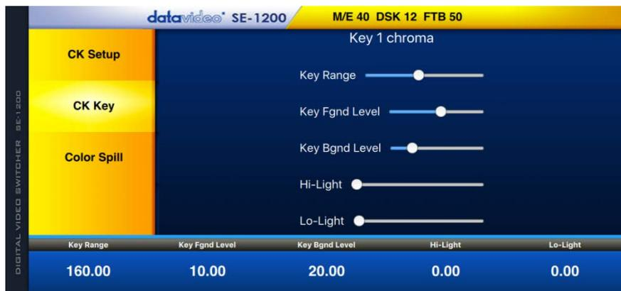
The Chroma Key control parameters and values are shown in the blue bar on the bottom of the screen. Users can control and adjust various parameters such as Key Range, Key Foreground Level, Key Background Level, Hi-Light and Lo-Light by using different sliders shown on the screen respectively.
