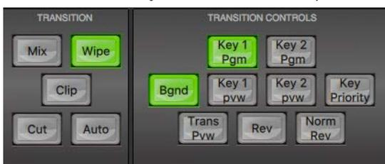
When the **Rev** button is **ON** then the selected transition will operate in the reverse direction only.
