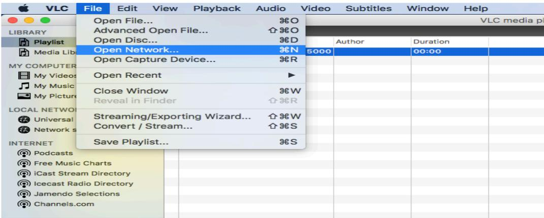
After entering into the “**Open Network**” option, input the streaming website address “tcp://192.168.100.101:5000” in the URL blank. After that, press the “**Open**” button and then the Multiview screen will be played in the VLC player window.
