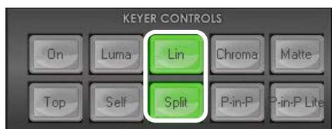
**Step 2:** We then choose the **Lin** or Linear and **Split buttons** from the **KEYER CONTROLS** panel to select a linear key.
