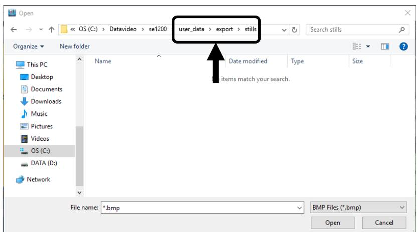
For each image exported, there will be two files, a thumbnail picture ending .mini and the full screen image ending .pic. These files can be then imported to another SE-1200 MU by pasting the files into the Import based stills folder on the second SE-1200 MU.
