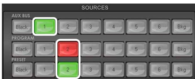
**Step 3:** Select the **foreground video** source with the subject or talent to be keyed. In our example, we want to use a green screen source connected to **Input 1** on the **Aux Bus Row**.
