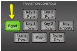
In order to mix between two video sources, first ensure the Background Transition or **Bgnd** button is ON / backlit green in the **transition controls** area of the user interface.
