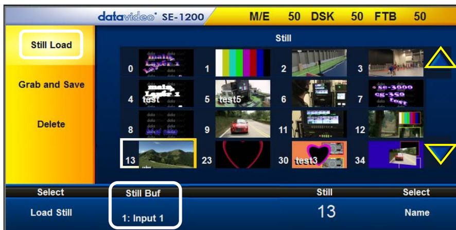
4. Change the **Still Buf option** in the lower row of options **to match the desired bus channel** that you wish to use to display the still image. In our example we have chosen **Input 1**.
