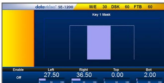
2. The Mask parameters are displayed along the bottom of the screen.
