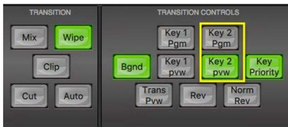
**Step 3:** Turn the Key 2 PIP effect on in the Multi view **Preview output** by clicking the **Key 2 PVW** button (backlit green) in the **Transition Controls** panel.
