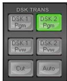
The labelled DSK 1 (Pgm/Pvw) or DSK 2 (Pgm/Pvw) buttons can be off or on. When a selected DSK button is green it is on and the active DSK result is seen in the multi view Preview video image.
