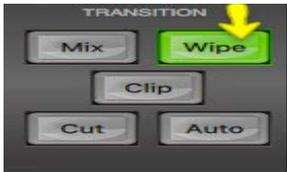
Clicking **Wipe** will select the current wipe transition in use when moving from the current video source on the Program row to the selected next source on the Preset row.
