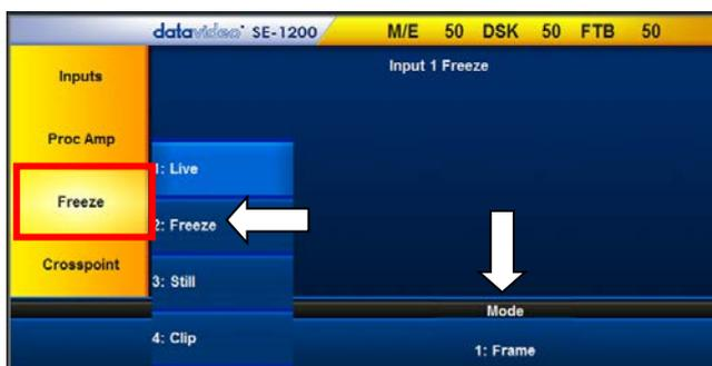
3. The Freeze parameters will then be displayed along the bottom row of the screen.
