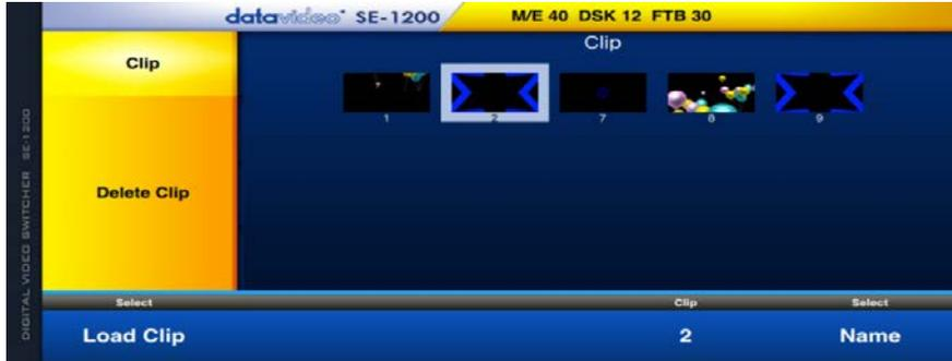
To load the clip, simply click on the **Clip** option and then select **“Load Clip”**. The clip is always loaded to input 6 so anything loaded to input 6 before will be replaced by the clip.
