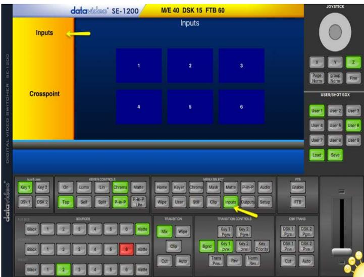
The physical input sources can be swapped around within the SE-1200 MU by using the **cross point** section of the **Inputs** menu.
