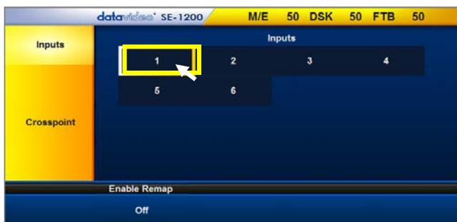
2. Six video input channel selection buttons will be displayed. **Click on the input channel button that you wish to Freeze.**
