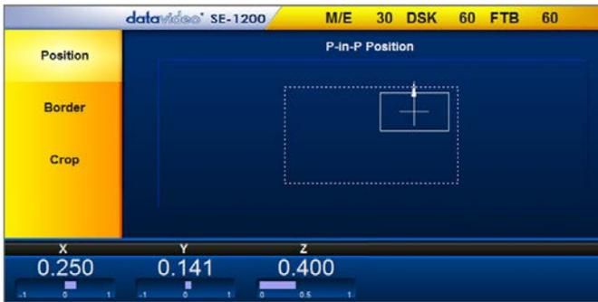
**Step 6:** PiP options displayed in the yellow menu area: **Position**, **Border** and **Crop**. The sections below will describe how Position, Border and Crop can be adjusted.
