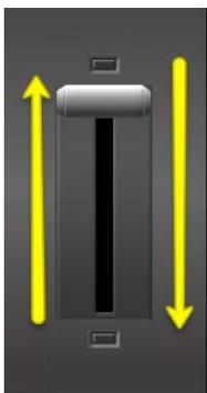
The timing of a **Wipe** transition can also be manually decided when moving the **T-Bar** or completed over a set duration when using the **AUTO** button.
