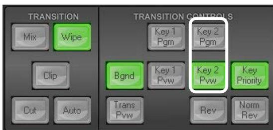
**Step 3:** Turn the Key 2 PiP effect on in the Multi view **Preview output** by clicking the **Key 2 PVW** button (backlit green) in the **Transition Controls** panel.
