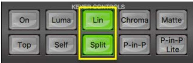
**Step 2:** We then choose the **Lin** or Linear and **Split buttons** from the **KEYER CONTROLS** panel to select a linear key.
