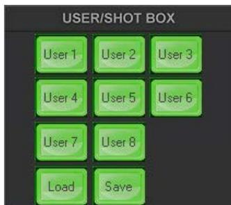
To load a previously saved SE-1200 MU Setup, simply click the **LOAD** button on the **USER/SHOT BOX** panel and an on-screen number pad will open.
