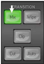
Pressing **Mix** will select a mix transition to use when moving from the current video source on the Program row to the selected next source on the Preset row.
