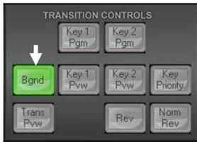
In order to mix between two video sources, first ensure the Background Transition or **Bgnd** button is ON / backlit green in the **transition controls** area of the user interface.
