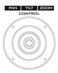
3. Use the joystick to zoom the frame and adjust its start position (fine border frame).
