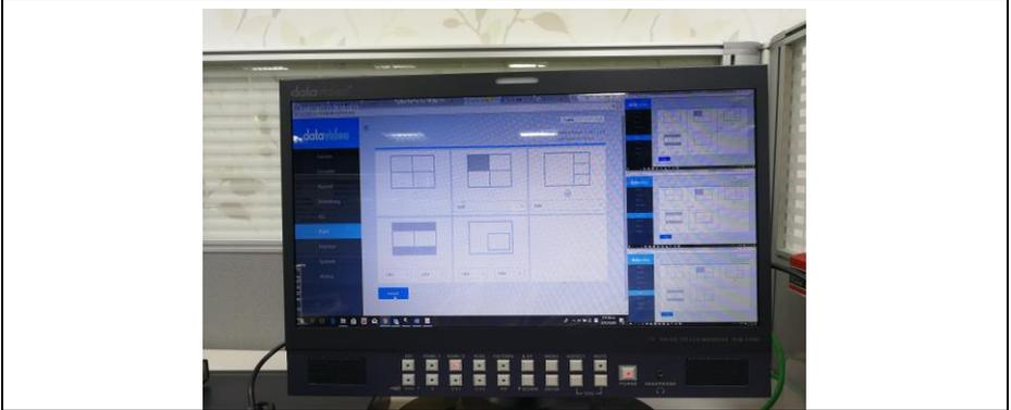
4. PBP (Picture By Picture): Click the PBP icon and select the desired two channels to be PBP and then press the submit button to apply.
