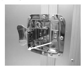
Undo each clasp by folding the wing nut out and then rotating it. The clasp can then swing free of the catch.
