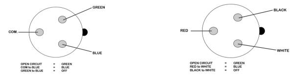
There is a 2m remote control cable supplied with the LD-1, this can be used in integrate into your chosen application. The diagram on the right above uses the colour coding of the supplied cable.
