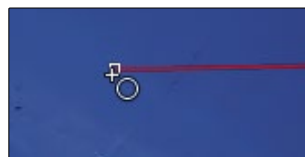
The close pointer is displayed when positioned over the first anchor point in a spline
