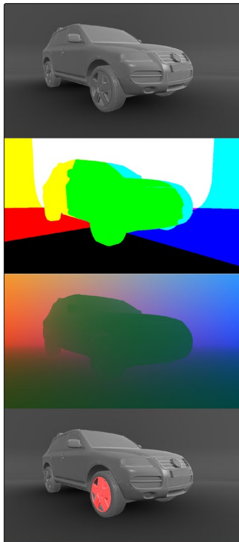
A World Position Pass Rendering of a scene with its center at (0,0,0). Actual image is on the left.
