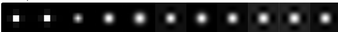
Different Resize Filters. From left to right: Nearest Neighbor, Box, Linear, Quadratic, Cubic, Catmull-Rom, Gaussian, Mitchell, Lanczos, Sinc, Bessel
