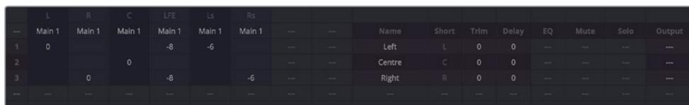
The Inputs/Outputs Table of the B-Chain preset window fully populated to assign inputs to outputs
